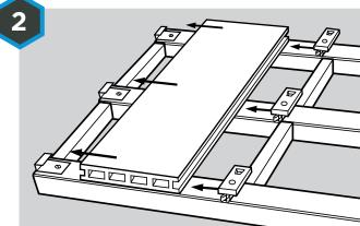
Place the first piece of decking on the timber frame with the decking running perpendicular to the joists. The first piece of deck may be secured with starter clips. Do not screw or nail through HD Deck® XS, use one Universal Clip and screw on every joist.
